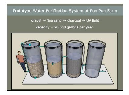
Here's an illustration done by my colleague of how the system will be configured, with gravel and sand filters to remove turbidity and microorganisms, and an optional germicidal UV unit for further disinfection at the point-of-use.
