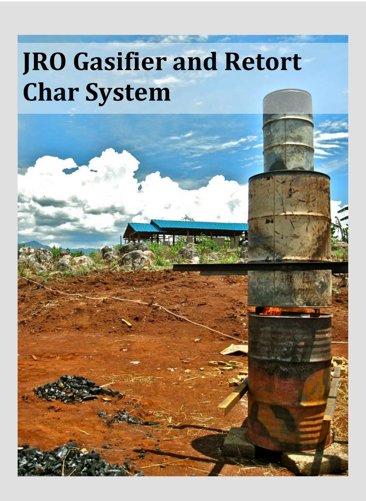
The purpose of this handbook is to show the construction and operation of a JRO ("Jolly Roger Oven") char manufacture system. The JRO costs \$50-90 to build, and uses the waste heat given off by a high temperature gasifier char oven (lower unit) to make a smaller batch of low temperature retort (upper unit) char. The high temperature gasifier char is ideally suited for water treatment applications and the low temperature retort char is excellent for use as cooking fuel.
