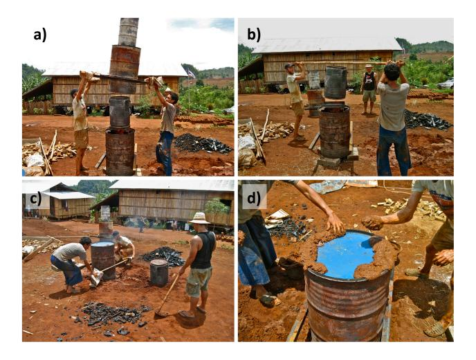
When all wood gases have been burned from the gasifier leaving only a faint blue flame, remove the chimney and set it aside (a). Remove the retort and place it lid-down into a mud pit to seal the slits and prevent ingress of oxygen (b). Remove the retort/chimney support and set it aside; place the lid on the gasifier and set the gasifier into the mud pit to seal the bottom (c). Seal the lid of the gasifier with mud (d). Allow retort and gasifier to cool at least 2 hours before removing char.
