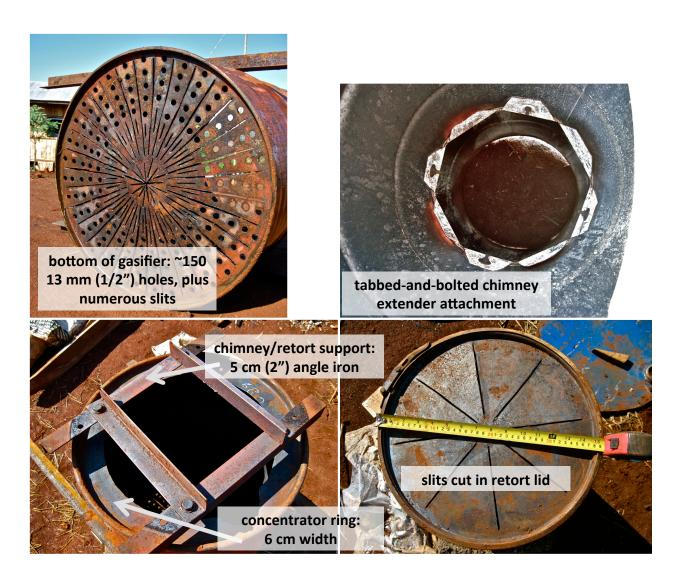
Using a drill and/or grinder, make as many holes as possible in the bottom of the gasifier drum without making it too weak. Cut two 60 cm and two 40 cm pieces of angle iron and bolt them together in a square configuration to make the retort/chimney support. Cut a 5-6 cm lip in the top of the gasifier drum to serve as a concentrator ring – this channels combusting gases into the chimney and prevents flames from escaping sideways out of the combustion zone.
