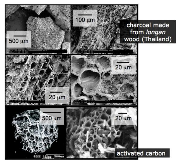
Scanning election microscope (SEM) images of *longan* charcoal and commercial activated carbon showing morphological similarities. (Charcoal SEM images courtesy of Carl Saquing, North Carolina State University.)
