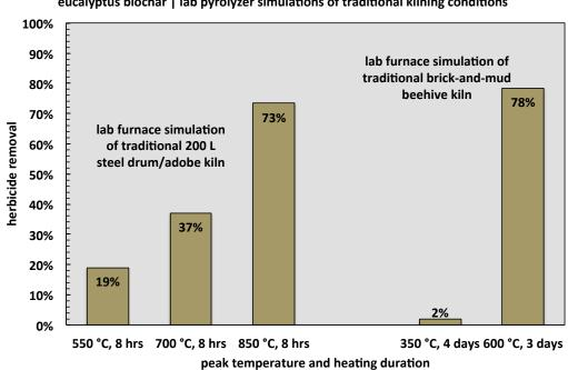
eucalyptus biochar | lab pyrolyzer simulations of traditional kilning conditions
