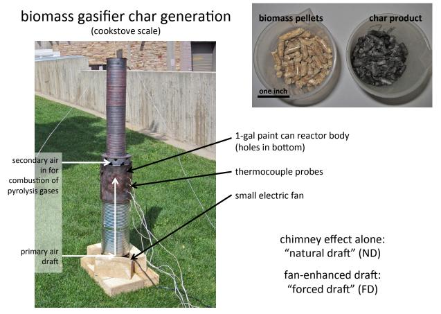
Cookstove-scale biomass gasifier char production unit. See Anderson et al. 2007,<sup>27</sup> Anderson 2010<sup>28</sup> and McLaughlin 2010<sup>29</sup> and 2011<sup>30</sup> for theory and detailed construction notes. (Thermocouple probes are for research purposes and may be omitted.)
