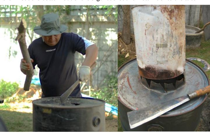
Use the machete and mallet to cut a hole out of the center of the pyrolyzer drum lid – leave a ring approx. 13 cm (5 in.) wide.
