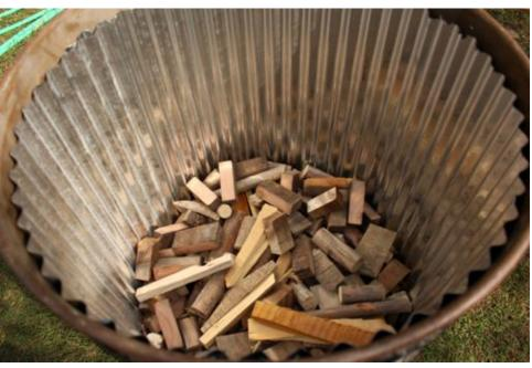
Fill the pyrolyzer drum with chopped scrap wood or tree prunings.
