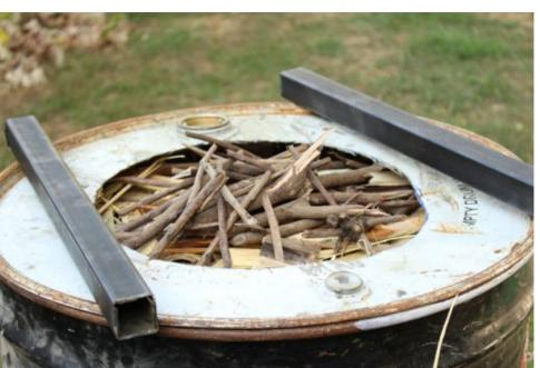
The feedstock should be packed tightly and uniformly. Use small pieces of wood or bamboo on top as kindling. Stack the chimney drum on top of the pyrolyzer drum as shown belowleft. Use the pieces of angle iron or square tubestock to create air gaps (1) between the pyrolyzer drum and the ground, and (2) between the drums.
