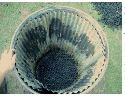
Cut the tin to fit inside the pyrolyzer drum as shown left.
