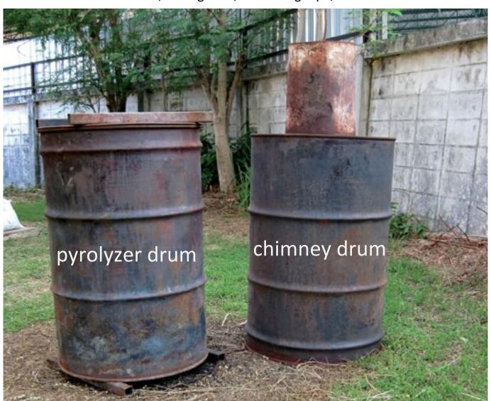
Use the machete and mallet to cut a tabbed hole in the top of the chimney drum. Cut the bottom out of the 5-gal bucket and install it onto the tabs.
