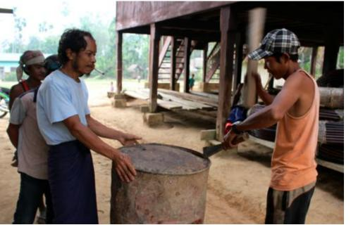
Cut out the bottom of the pyrolyzer drum leaving a 3-4 cm (1-1½ in.) lip as shown left and bottom-left.
