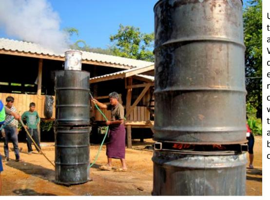
Use plenty of water to quench the char and cool the drums. When the upper drum is cool enough to handle, remove it and continue pouring water on char until there's no steam and all char has been thoroughly cooled.
