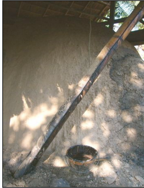
Wood vinegar collection from kiln chimney.
