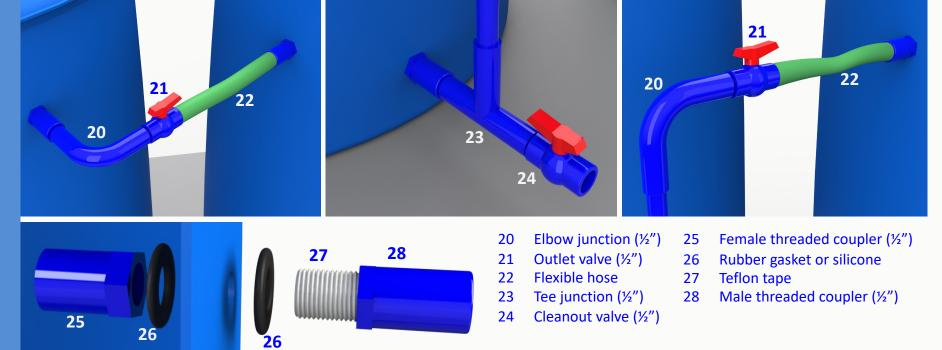
Cut holes in tanks manually with a pocket knife, or using a drill and hole saws: 20 mm for 1% fittings, and 48 mm for 1% fittings.
