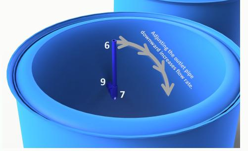
The maximum flow rate through the system is limited by the slow sand biofilter.
